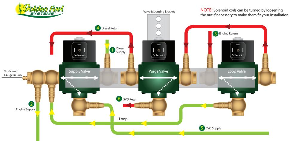
NOTE: When assembling the banjo fittings, the rubber centered washers go next to the valve body and the copper washers go on the end of the Banjo bolts.
