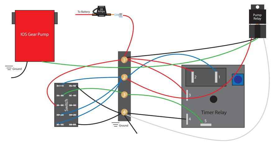
NOTE: Turning the blue knob on the delay relay clockwise will increase the time the pump stays on (Aprox. 6min maximum).
